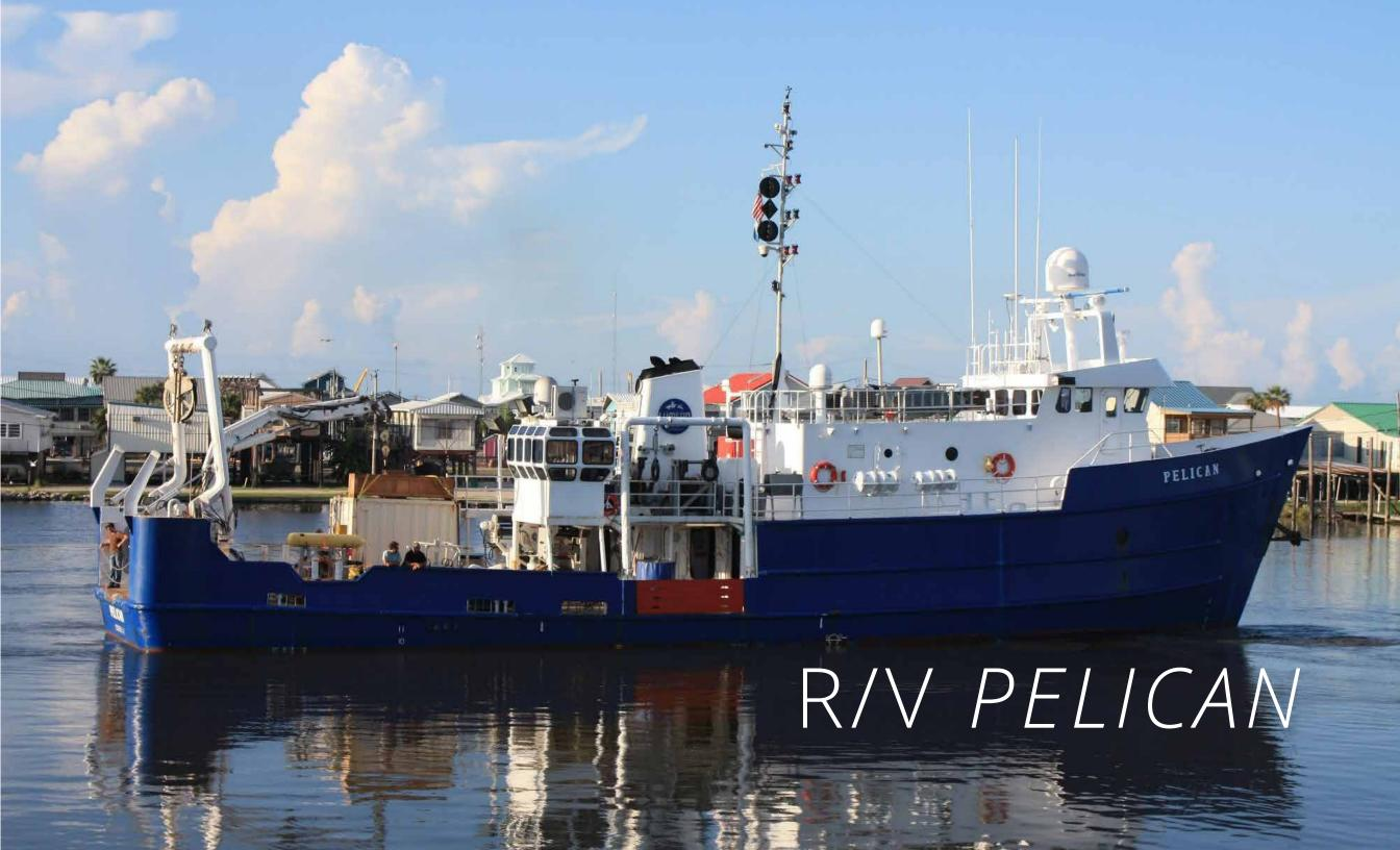
has a long track record of successful scientific research including: trawling, large box core sampling, thirty foot piston cores, shallow seismic surveys, ROV operations, buoy deployment and recovery, and hydrographic casts with CTD-rosette systems.
