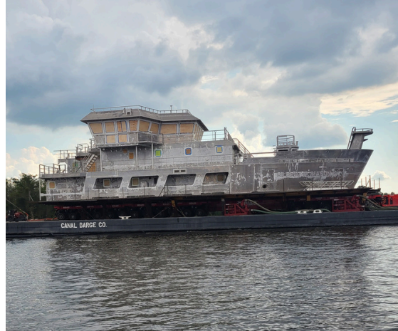
The superstructure of R/V Gilbert R. Mason in transit from Amelia to Houma
